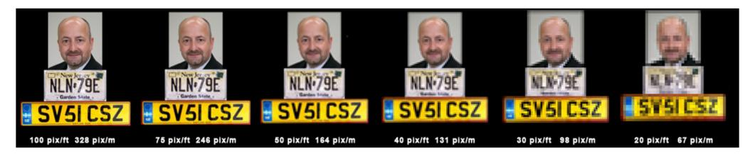
Reference images are captured under ideal conditions. Poor lighting, increased compression, or use of a lower quality lens will affect the quality of the images captured.
